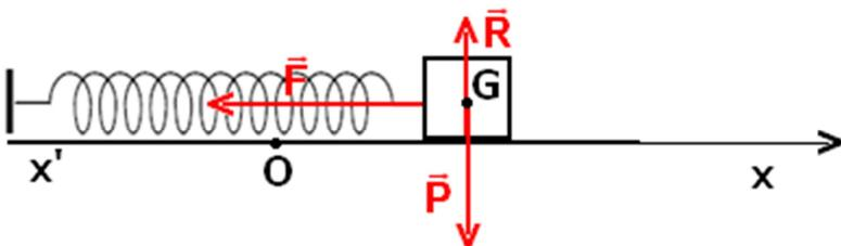
$$\left( \frac{k}{m} - \frac{4\pi^2}{T_0^2} \right) = 0 \Rightarrow T_0 = 2\pi\sqrt{\frac{m}{k}}$$
